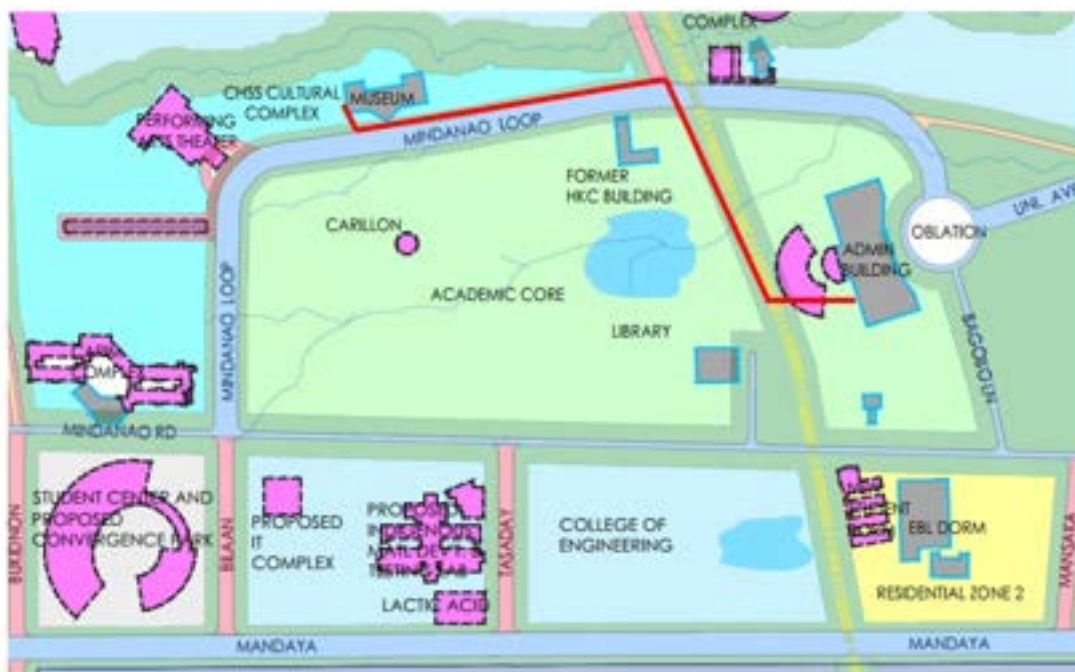
8-CORE FOC SM Aerial installation Using existing poles
