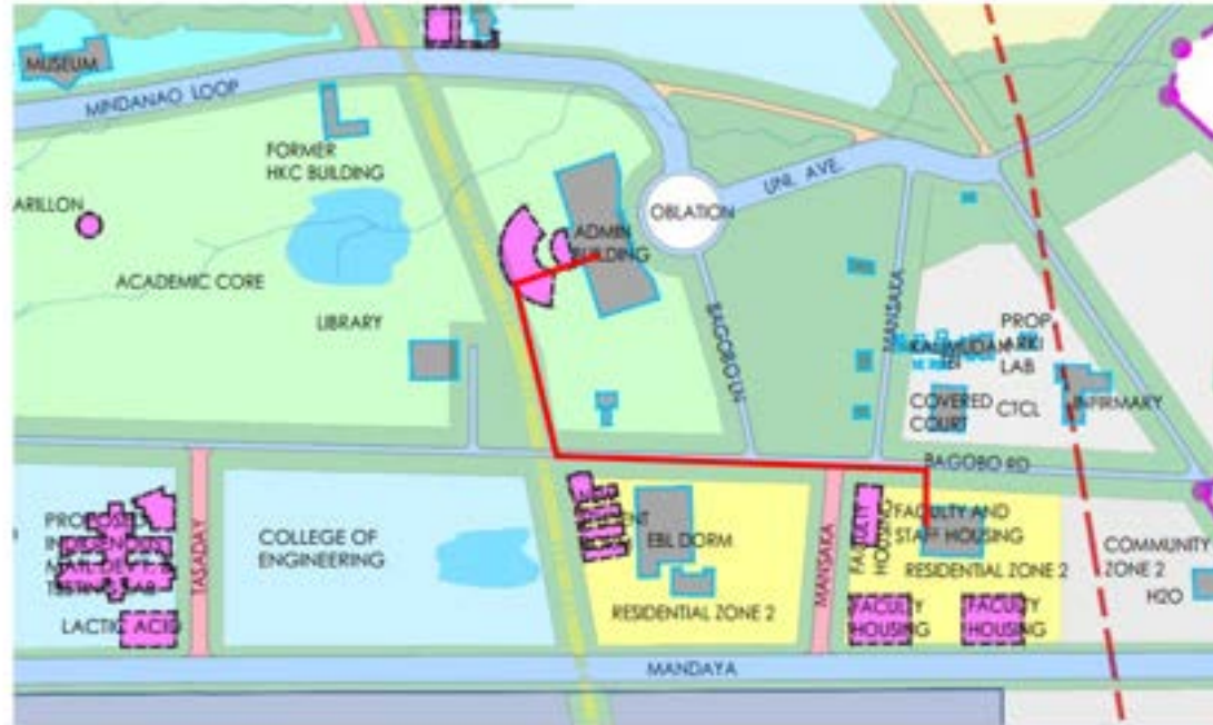
8-CORE FOC SM Aerial installation Using existing poles
