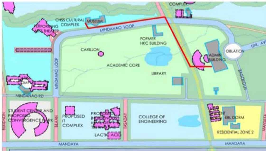
8-CORE FOC SM Aerial installation Using existing poles
