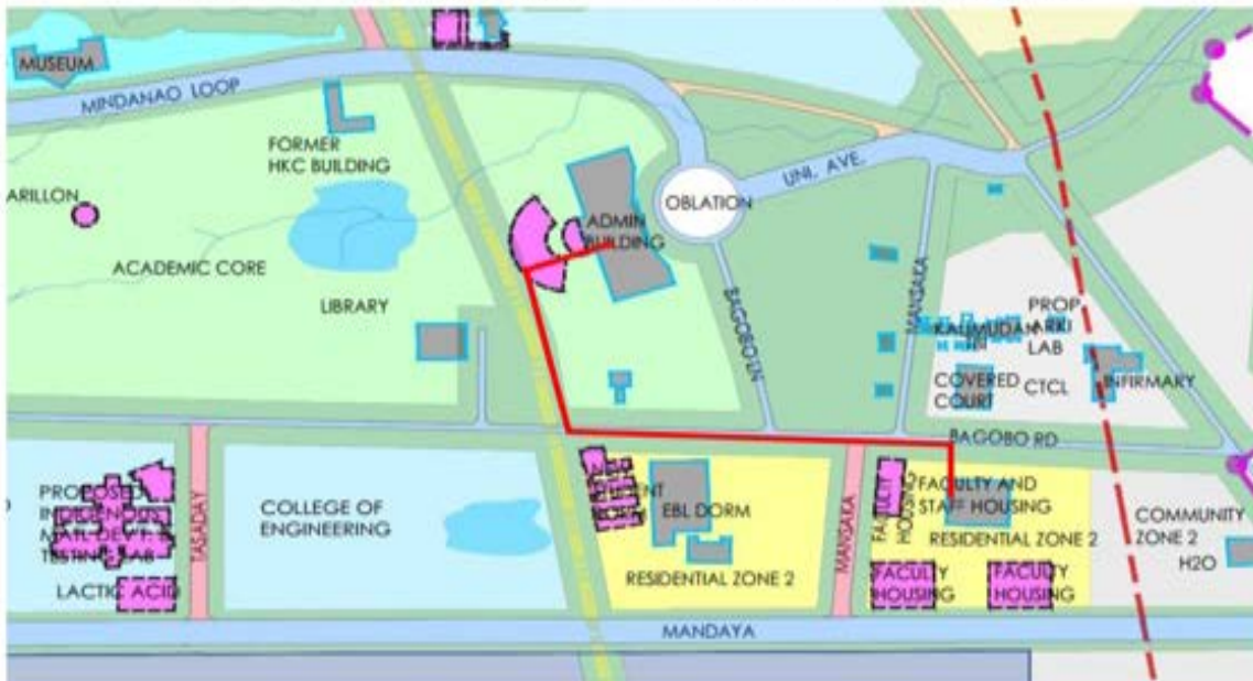
8-CORE FOC SM Aerial installation Using existing poles
